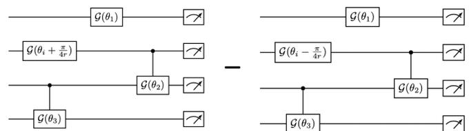
FIG. 4. Parameter shift rule. Same circuit is run twice with shifted parameters to calculate the gradient for 1 gate with respect to its variational parameter. This procedure is repeated for every gate for which a gradient needs to be calculated.
