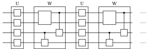
FIG. 3. General structure of hardware-efficient ansätze.  $U$  layer contains only single qubit gates whereas the  $W$  layer contains two-qubit entangling gates.
